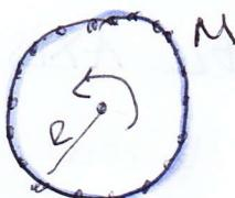
$$I_{\text{ring}} = M R^2 \quad (\approx \text{hollow cylinder})$$
