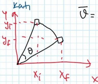
$$\bar{v} = \frac{\Delta X}{\Delta t} = \frac{X_f - X_i}{\Delta t} = \bar{v}_x$$
