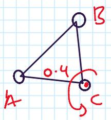
$$I_C = m_A r_A^2 + m_B r_B^2 \neq 0 = (0.3)(0.4)^2 + (0.1)(0.3)^2 = 0.057 \text{ kg m}^2$$
