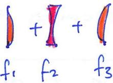
$\frac{1}{f_1} + \frac{1}{f_2} + \frac{1}{f_3} = \frac{1}{f_{\text{eş}}}$   $f_{\text{eş}} = ?$
