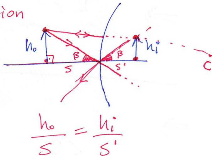
$$m = -\frac{s'}{s} \quad \begin{array}{l} \times \\ \times \\ \times \end{array} \quad \begin{array}{l} M > 0! \\ \text{düz} \\ M < 0 \\ \text{ters!} \end{array} \quad \begin{array}{l} h_o \uparrow \\ \downarrow h_i \end{array}$$
