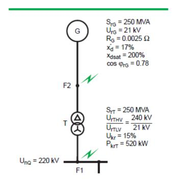
The single-pole short circuit current is to be calculated at the end of the line, considering the zero-sequence resistances. The data are given in Figure
