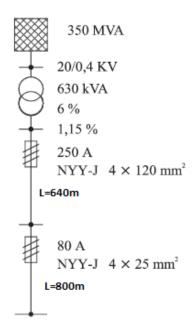
In the electrical installation of a building the following data are known (Figure ). Calculate all required short circuit currents and check the cut-off con-P4) ditions.
